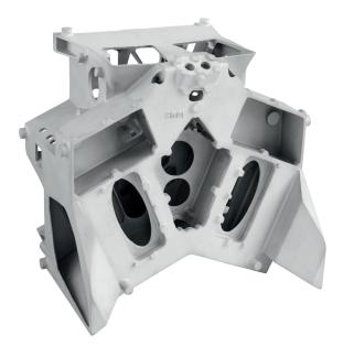
The TNO Sinplex-Casting – winner of the Aluminum Award 2014 / category "Aerospace and Automotive" – is an ultra-thin-walled miniaturised and extremely lightweight navigation subsystem for future space missions. The casting with its complex structure gets its particular characteristics by being produced with the SOPHIA-process.
