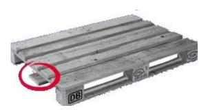
More than two bottom or top edge planks are so severely split that more than one nail or screw shaft is visible.
