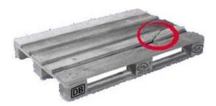
A block is missing or is split in such a manner that more than one nail is visible.
