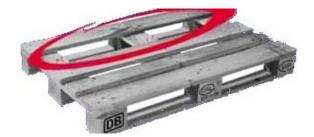
A board is transversely or diagonally broken.
